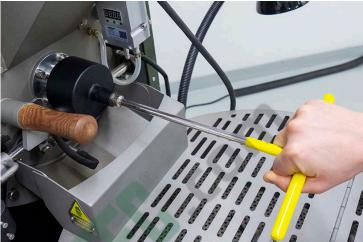
1. Use socket tool to unlock locking ring. Turn clockwise to lock and counter clockwise to unlock. Unlock it with two complete turns to allow room for adjustment.
