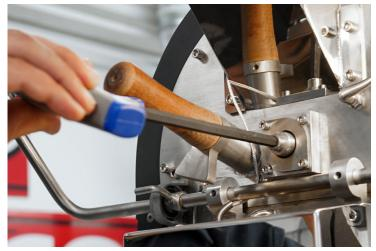
MANUAL DRUM TURNING/COOLING (above): In case of power outage, use included hand crank (left) to turn drums from rear shaft access on 2kg roasters and above until roast is safely cooled. For roasters 2kg and smaller (right), use an 8mm Allen wrench (not included) to turn drum shaft from the front. Additionally, spraying water on to the roast through the tryer hole may help cool the roast faster.
