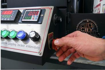
EMERGENCY STOP (above): The emergency stop button is either located on the back of your roaster or the right side of the control panel. Once pressed, it will disable all fans, motors, and gas flow.
