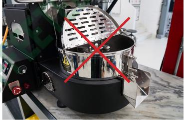
COOLING TRAY COVER (above): Cooling tray arms will NOT rotate if the cooling tray cover is open or removed or the sensor cable is unplugged.
