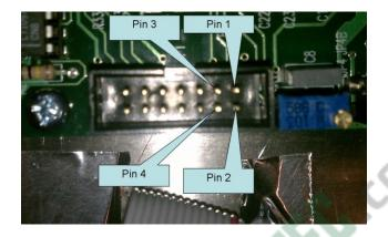
Short pins 1 and 2 using a conductive screwdriver. You will hear the unit click on and the LCD will now show a reading. You have just turned the unit on.
