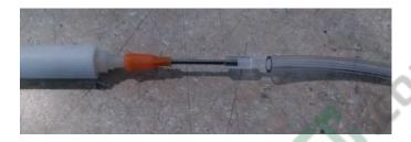
Also, make sure that the nitrogen has been flowing for at least 30 seconds to flush out any other air that may have been in the tubing.
